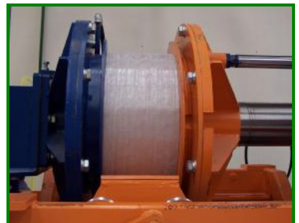
Hydraulic tests of couplings
