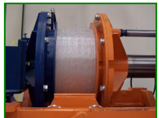
Hydraulic tests of couplings
