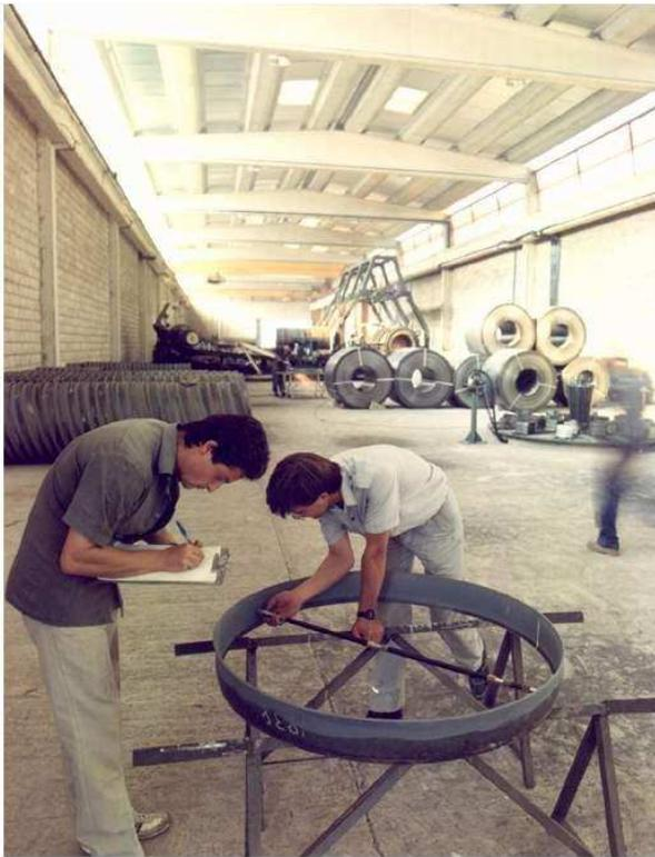
**Control dimensional cabezal expansionado**
